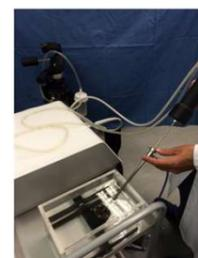
Pic.1: Set-up: Stones placed in a hemispherical silicone support inside a water container
