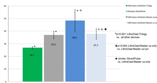
Fig. 1: Average Clearance Time (10mm<sup>3</sup> cubes / 15:3 ratio)
