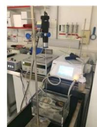
Pic.3: Set-up: Drilling Speed Test
