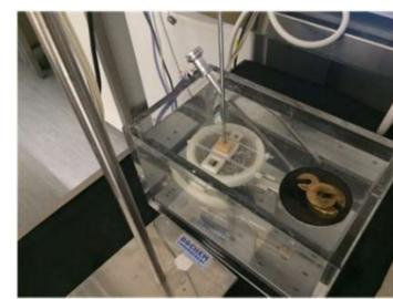
Pic.4: Set-up: Stones placed in an under-water balance with a 450g weight placed on the other side
